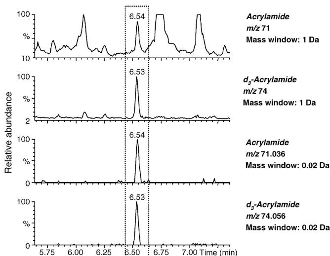
Fig. 3. GC–HRTOF MS analysis of acrylamide in crisp bread samples (450  $\mu\text{g kg}^{-1}$ ) under conditions of different mass window settings (1 and 0.02 Da) for extraction of target ions.
