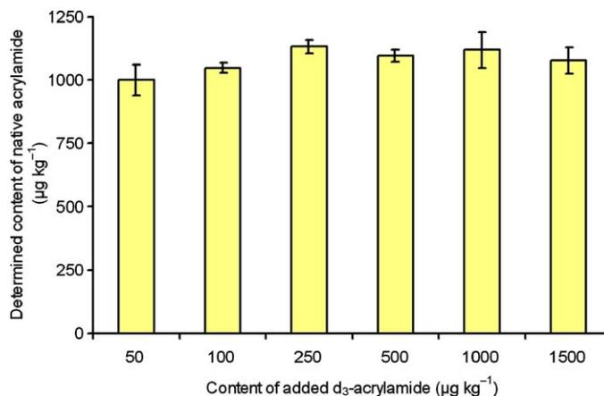
Fig. 4. Results of native acrylamide determination in bread extract to which increasing amounts of  $d_3$ -acrylamide (internal standard) were added for quantification (error bars are  $\pm$  S.D.;  $n = 3$ ).
