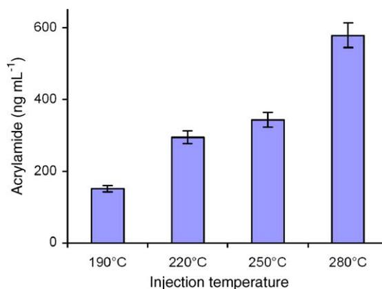
Fig. 1. Formation of acrylamide in the hot splitless GC injector (error bars are ± S.D.; *n* = 3). A 1 μL of aqueous solution of L-asparagine and D-glucose (each 50 μg mL<sup>-1</sup>) injected. d<sub>3</sub>-Acrylamide used for quantification.
