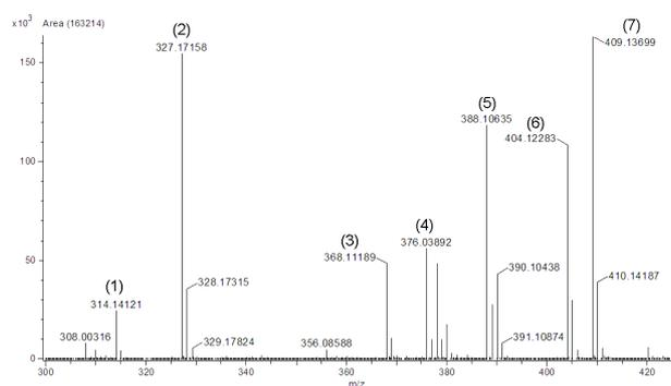
Fig. 1. Dart positive mass spectrum of wheat grain extract spiked with strobilurins ( $240 \text{ ng g}^{-1}$ ) and prochloraz ( $250 \text{ ng g}^{-1}$ ); (1) Kresoxim methyl, (2) Dimoxystrobin, (3) Picoxystrobin, (4) Prochloraz, (5) Pyraclostrobin, (6) Azoxystrobin, (7) Trifloxystrobin
