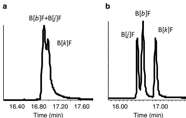
Fig. 3. GC separation of “critical” PAH isomers employing (a) (5%-phenyl)-methylpolysiloxane (30 m × 0.25 mm × 0.25 μm) and (b) 50% liquid crystalline–methylpolysiloxane (10 m × 0.18 mm × 0.1 μm). Quadrupole mass analyser used for detection ( $m/z$  252 displayed).
