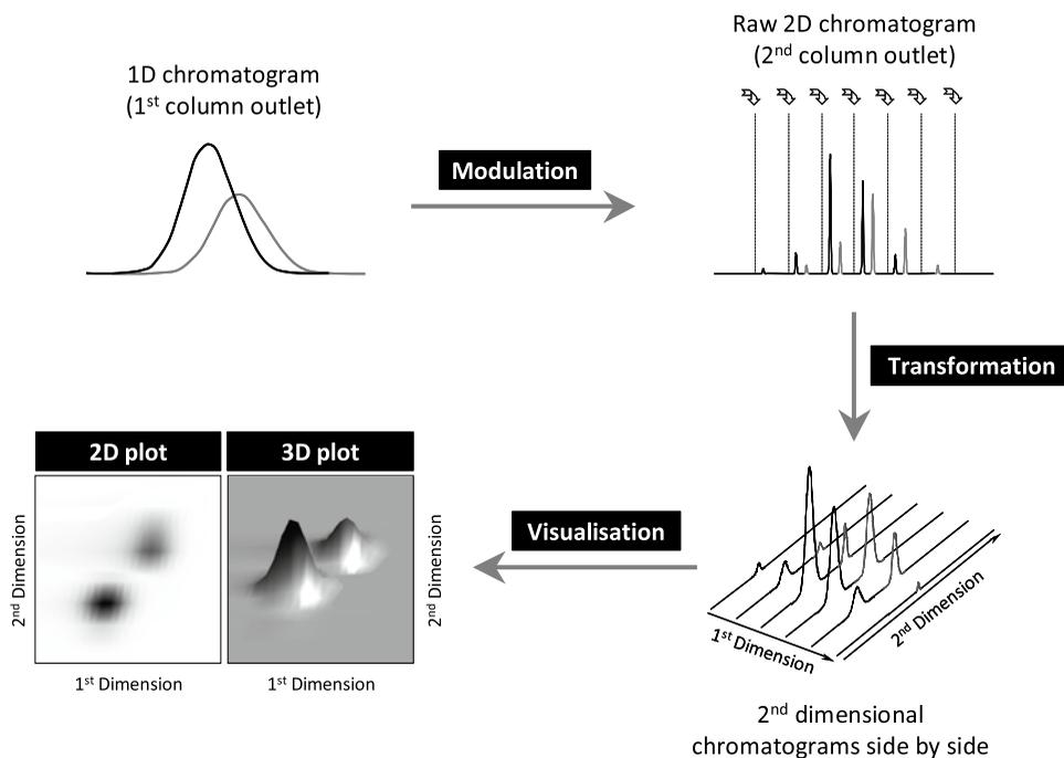
Fig. 4. Generation and visualisation of a GC  $\times$  GC chromatogram.
