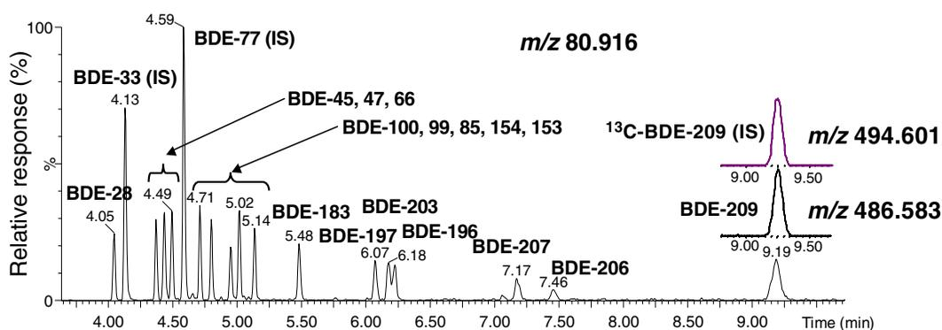
Fig. 2. LPGC–HRTOFMS chromatogram of standard solution of PBDEs detected in NCI mode (BDE-28, 47, 49, 66, 85, 99, 100, 153, 154, 183, 196, 197, 203 at a concentration of 0.5 ng/mL; BDE 206, 207, 209 at a concentration of 1 ng/mL; BDE 37 and 77 at a concentration of 5 ng/mL, and  $^{13}\text{C}$ -BDE-209 at a concentration of 50 ng/mL; 1  $\mu\text{L}$  injected). The target ions (bromine  $[\text{Br}]^-$  with exception of BDE 209) were extracted using a narrow 0.05 Da mass window.
