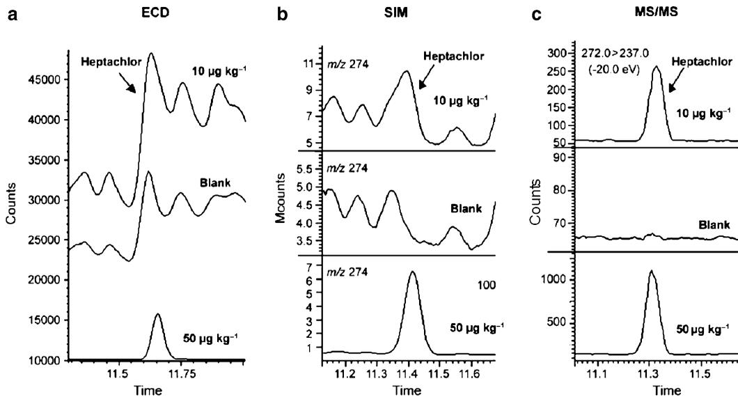
Fig. 8. Comparison of selectivity between (a) electron-capture detector (ECD), (b) selected ion monitoring (SIM) of a single quadrupole, and (c) tandem MS (MS/MS) of a triple quadrupole for heptachlor at 0.01 mg/kg in fish oil. Chromatograms of the corresponding blank extract and a higher matrix-matched standard are provided for contrast and identification (Reproduced from (40) with permission from Elsevier).
