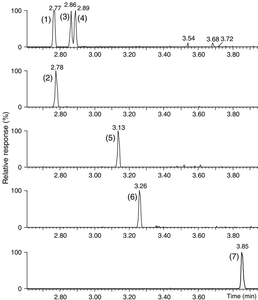
Fig. 1. PTV-LPGC-El-HRTOFMS chromatogram of selected OCPs at a concentration of 0.01 mg/kg fish oil extract. The target ions were extracted using a 0.02 Da mass window. (1)  $\alpha$ -HCH ( $m/z$  180.938), (2) HCB ( $m/z$  283.810), (3)  $\beta$ -HCH ( $m/z$  180.938), (4)  $\gamma$ -HCH ( $m/z$  180.938), (5) heptachlor ( $m/z$  271.810), (6) aldrin ( $m/z$  262.852), (7)  $p,p'$ -DDT ( $m/z$  235.008).
